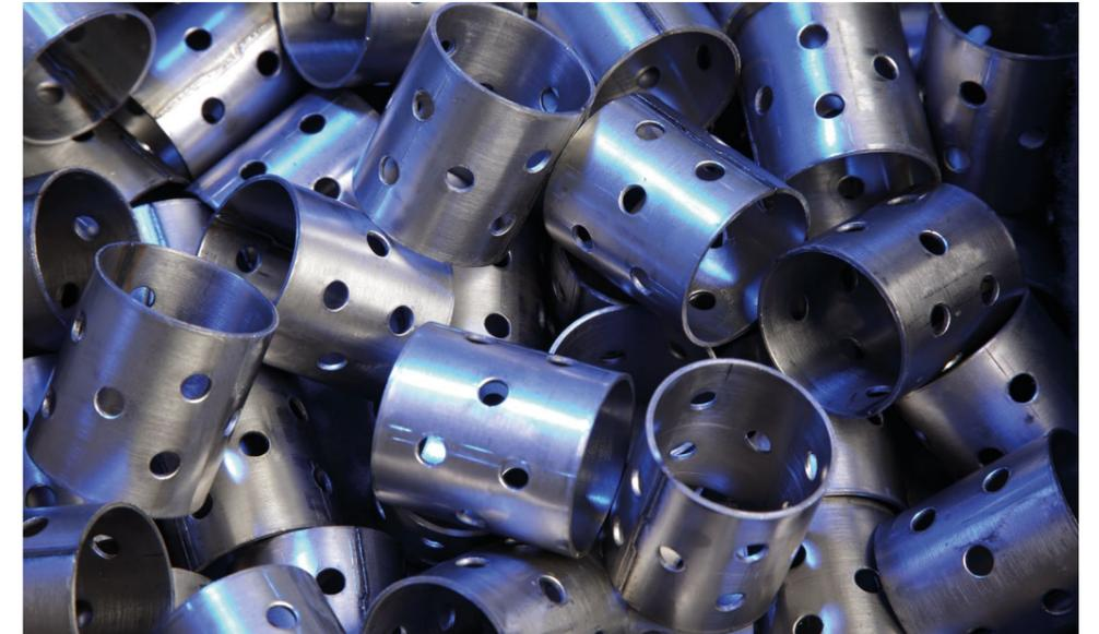
The manufacturing of rings, bushes and sleeves can be carried out efficiently and economically with the aid of punching-bending technology. Here a strip of metal is cut to length and bent around a core. The two ends stand in front of one another in the form of a slot or are joined by clinching.
